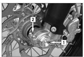
To install the front wheel, lift it into the fork, position and mount the axle shaft [3]. Mount the collar nut [1], tighten the clamping screws [2] on the right fork leg axle passage to prevent the axle shaft from turning and tighten the collar nut to 40 Nm.
